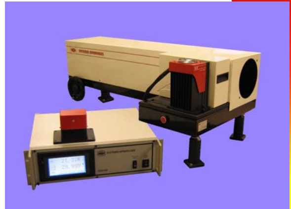
Collimator assembly with blackbody controller
