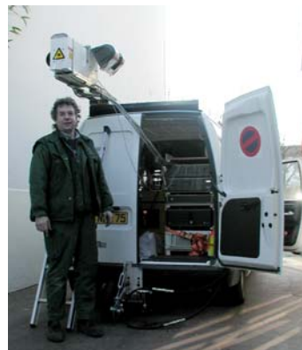
Inspection vehicle for road tunnels
